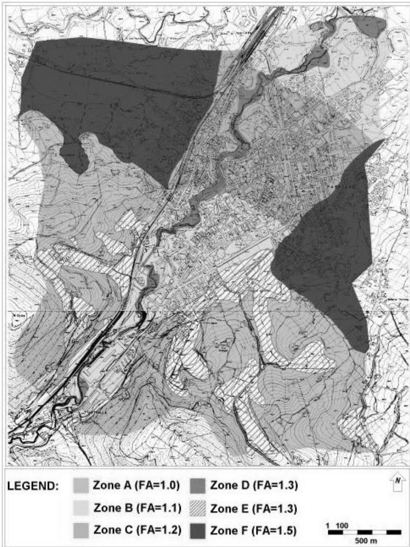
Fig. 7.4. Fabriano zonation map; FA represent an amplification coefficient, eventually used by the designer as multiplicative factor of design forces (after Marcellini et al., 2001a, Reproduced by permission of Italian Geotechnical Journal - Patrono Editore).
